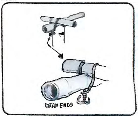
Finally secure the middle laths. Place these equidistant from the top and bottom laths. If a drill and screws are on site, then set screws into the poles to secure each lath firmly in place.
