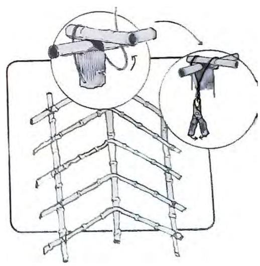
Secure the beams to the poles with wire. Drilling in a screw in the top of the pole, just under the notch, can help in fixing the wire. If fresh bamboo is being used, it will contract after exposure to sun. This often causes the fitting to loosen. Be sure to recheck the
