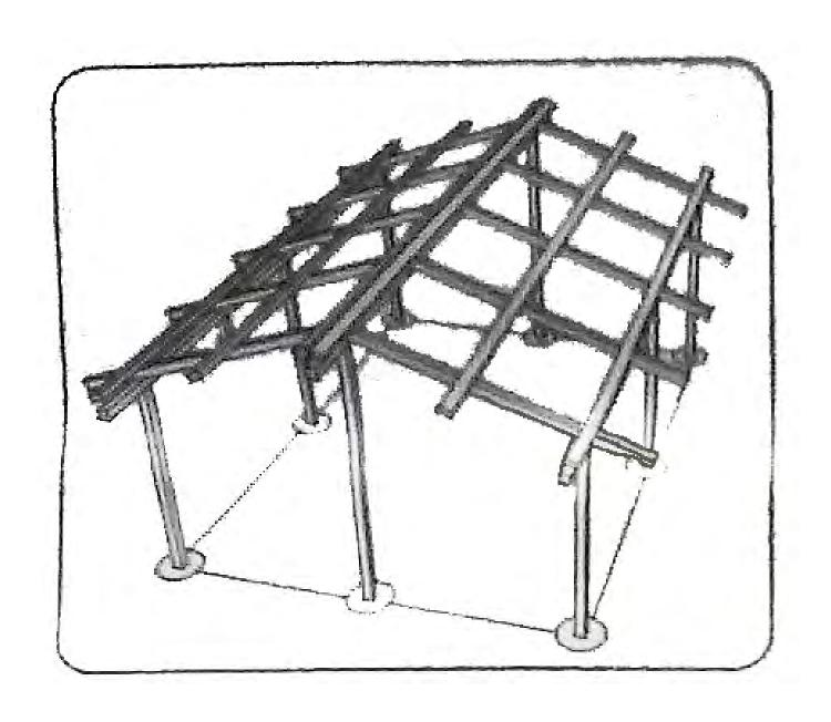
Next secure the bottom laths. They should be secured about 8 inches down from the bottom beams, or at least at the bottom beam.
